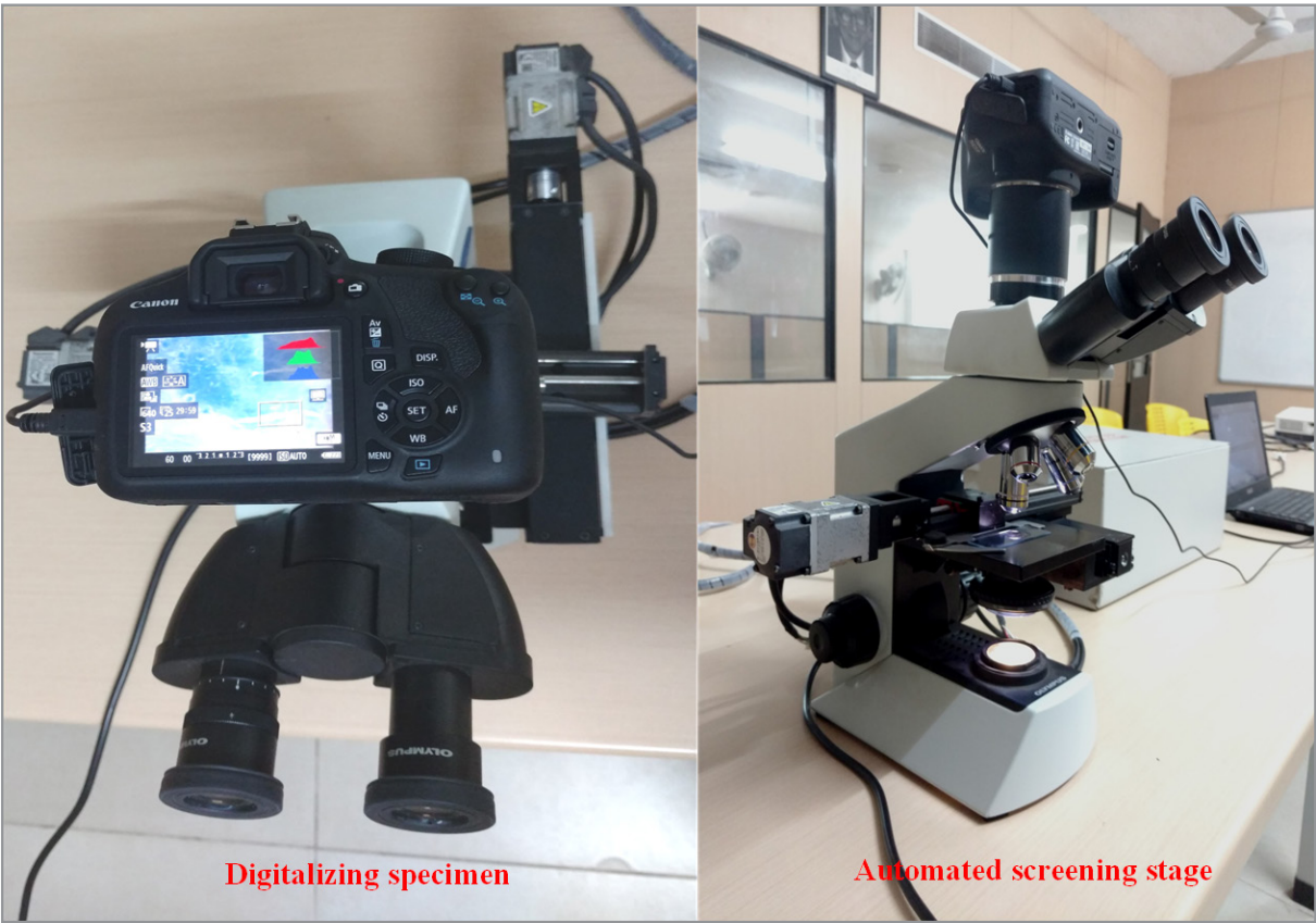
Figure 2. Automated digitalization of specimen using programmable microscopic stage.
